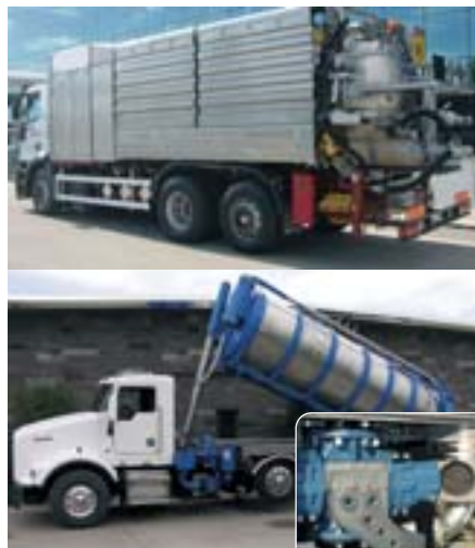
• Mobile units for the suction of dusts and/or liquids Vacuum blower unit: TRB-DV
