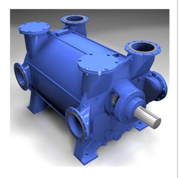
The 2BE4 pumps allow efficient operation over the entire vacuum range without the need to change the pump's internals. When equipped with a center shroud, split vacuum operation up to 12 in. Hg (400 millibar) differential can be achieved. Large inspection ports allow easy access to pump internals for inspection and maintenance.
